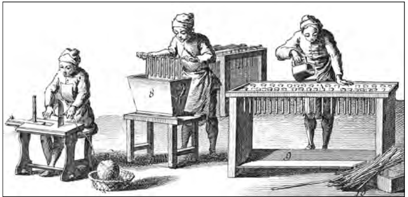
Sketch from Denis Diderot's L'Encyclopedie , originally published in the 1750s. The man on the left is cutting wicks to the desired length while the man in the center dips them into hot tallow. The chandler on the right is pouring hot wax into a mold.
